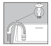
In a sink drain pipe branch. This branch must be above the trap so that the bend is at least 60 cm above the around.
